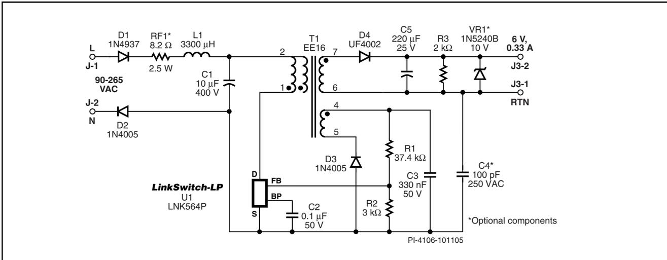
Figure 5. 6 V, 330 mA CV/CC Linear Replacement Power Supply.
