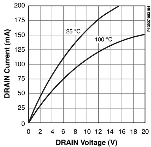
Figure 17. Output Characteristics.
