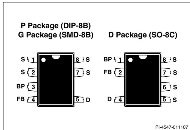
Figure 3. Pin Configuration.
